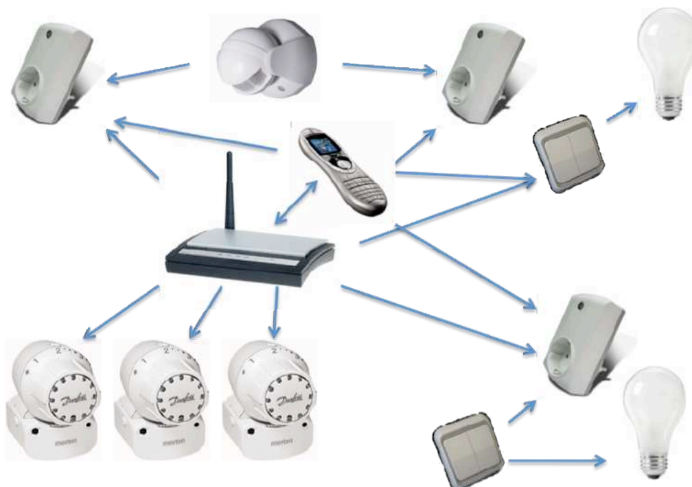
Figure 3.19: Z-Wave Network with multiple controllers
