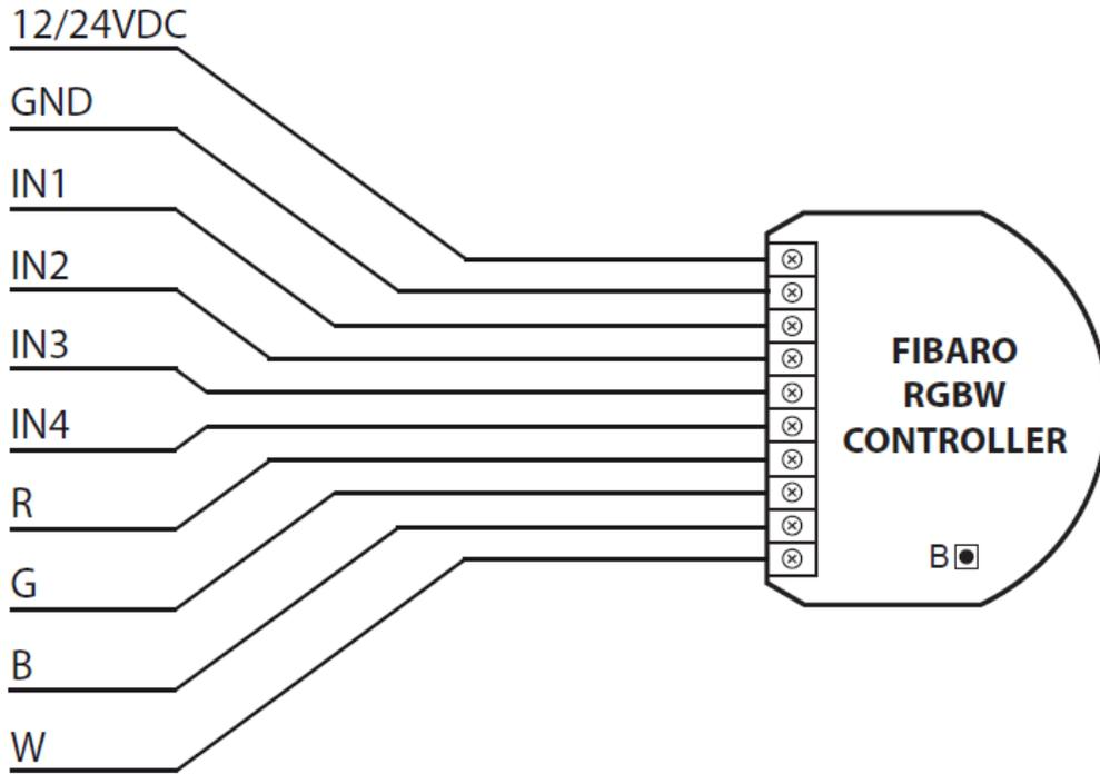
Figure 3.34: Fibaro RGBW Controller - Terminals description
