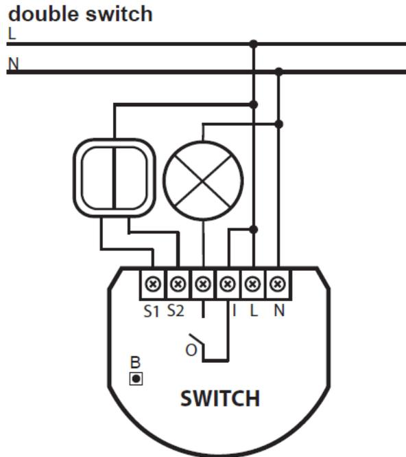
Figure 3.22: Double switch, Relay Switch 1x3kW wiring diagram
