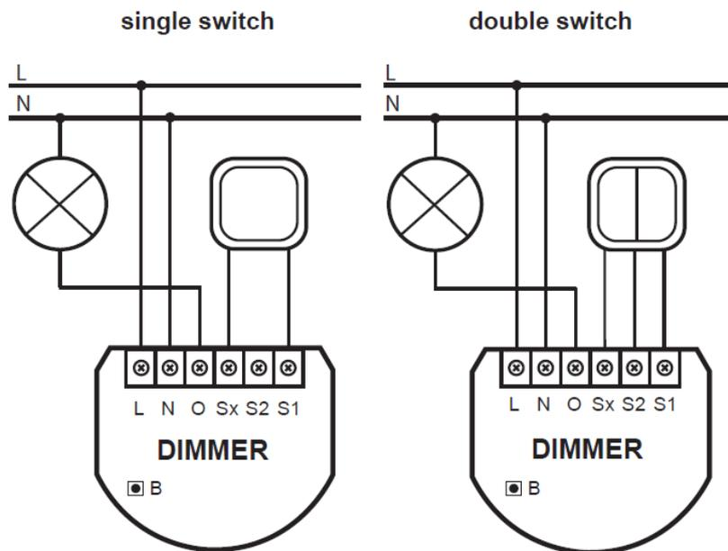
Figure 3.9: Dimmer wiring diagram - 3-wire connection
