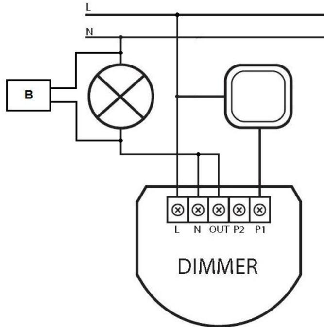
Figure 3.31: Wiring diagram - Bypass
