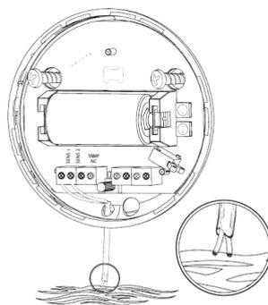
Figure 4.19: Flood sensors contacts extended with a wire
