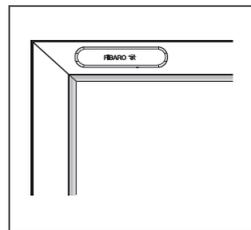
Figure 4.13: Door Window Sensor - correct sensor installation
