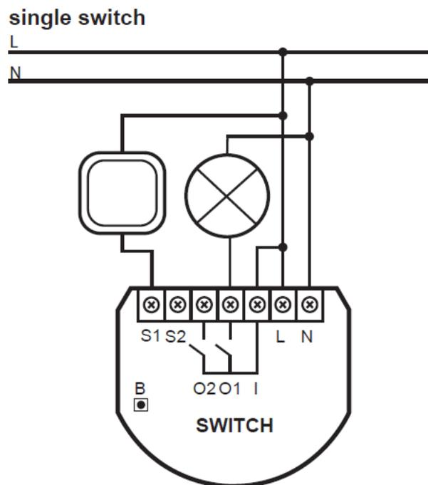
Figure 3.14: Single switch, Relay Switch 2x1,5kW connection diagram
