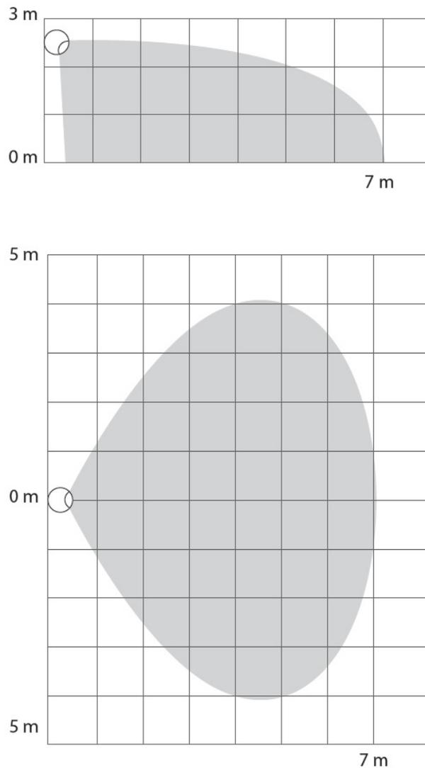
Figure 4.26: Fibaro Motion Sensors motion detection area
