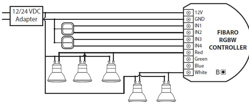
Figure 3.35: Fibaro RGBW Controller - Connecting halogen lighting
