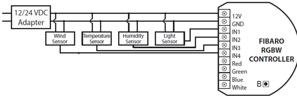
Figure 3.36: Fibaro RGBW Controller - 0-10 V sensors wiring diagram
