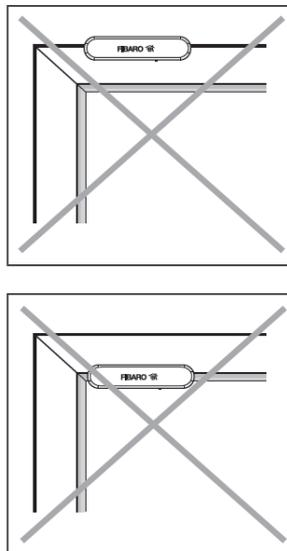
Figure 4.14: Door Window Sensor - incorrect sensor installation
