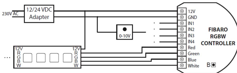
Figure 3.38: Fibaro RGBW Controller - RGBW strip 0-10V potentiometer wiring
