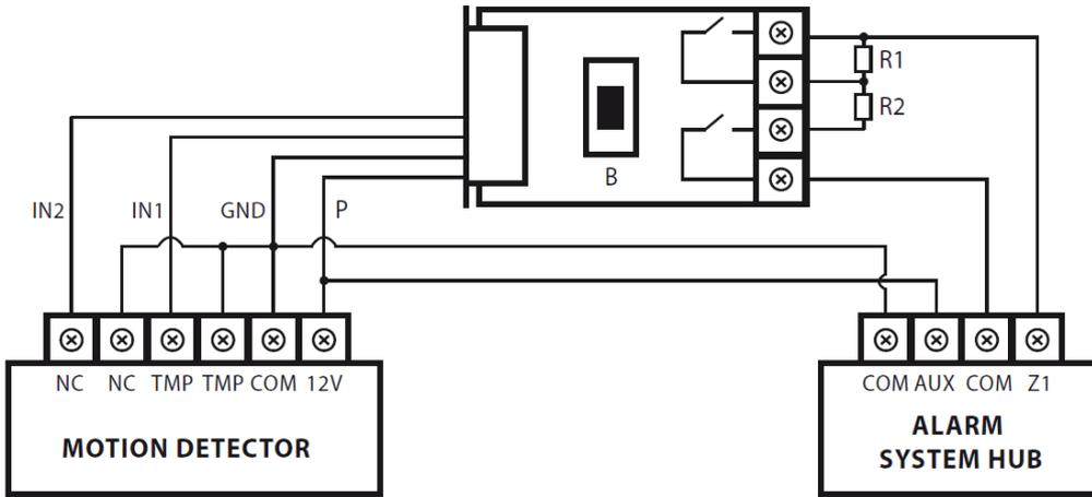
Figure 4.4: Universal Binary Sensor, parametric alarm line
