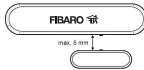
Figure 4.12: Door Window Sensor - correct positioning of the sensor and the magnet
